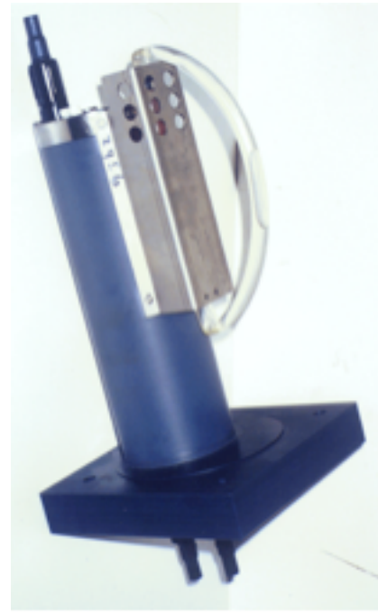
Electronics and sensor module of the SBE-21 thermosalinograph
